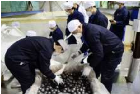
Workers inspect the spherical fuel elements prior to their loading (Image: CNN)
