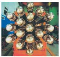
**Fig. 28.**Test facility of He-He heat exchangers in FZ-Jülich laboratory.
