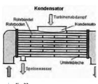
chematic of a turbine condenser.
