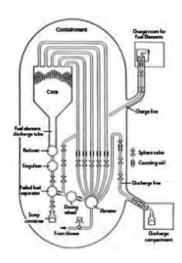
**Fig. 6.**Fuel cycle of pebble bed transportation system.
