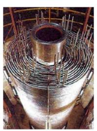
**Fig. 29.**Manufacturing of the THTR steam generator.
