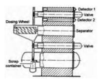
**Fig. 5.** View into the core of the AVR.
