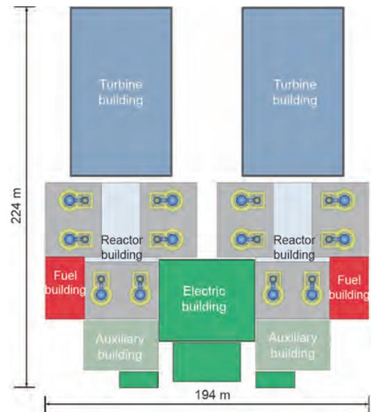
Fig. 6. The 2 × 600 MW<sub>e</sub> HTR-PM multi-modules plant.
