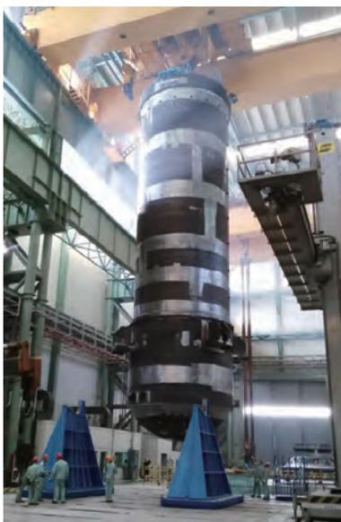
Fig. 4. Manufacture of the HTR-PM reactor pressure vessels by the Shanghai Electric Corporation; status as of September 2015.
